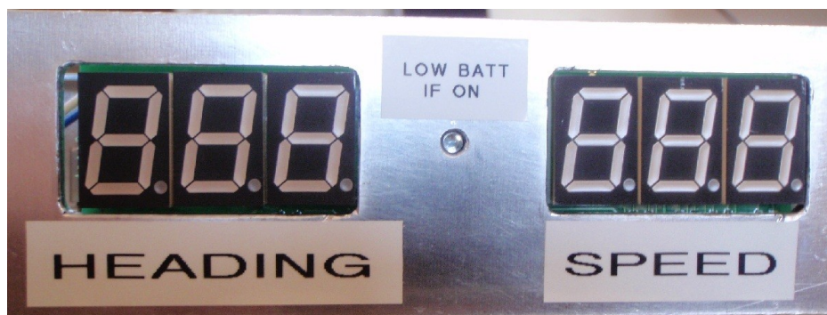
Front panel indicators – Heading, Speed, and battery/connection LED
