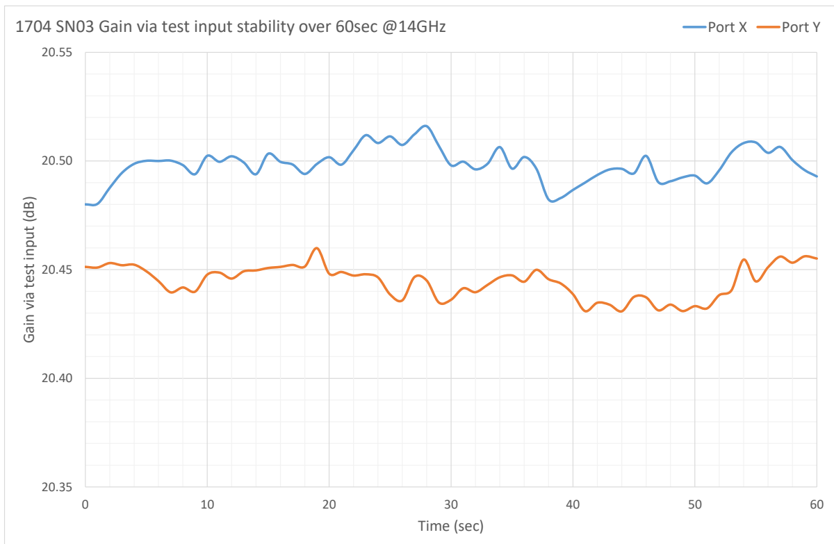
Figure 3-10: Gain via test input stability over 60sec (1 sample per sec) @14GHz
