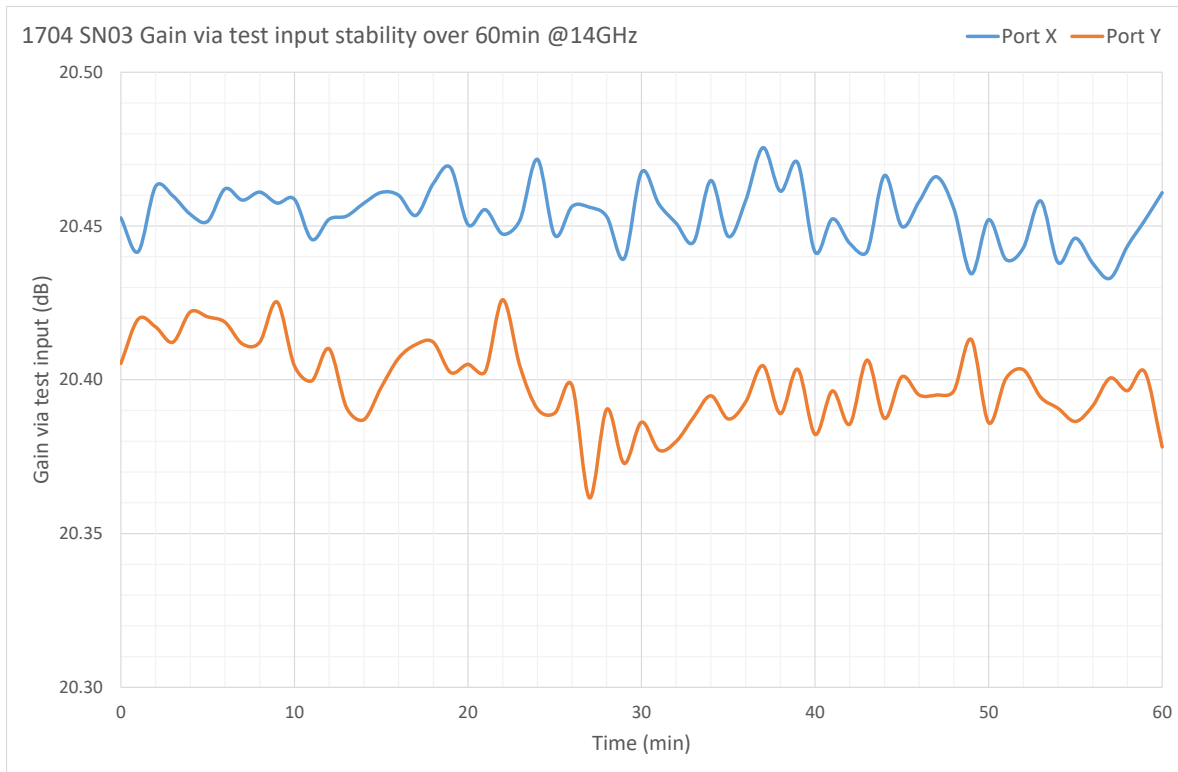
Figure 3-7: Gain via test input stability over 60min (1 sample per min) @14GHz
