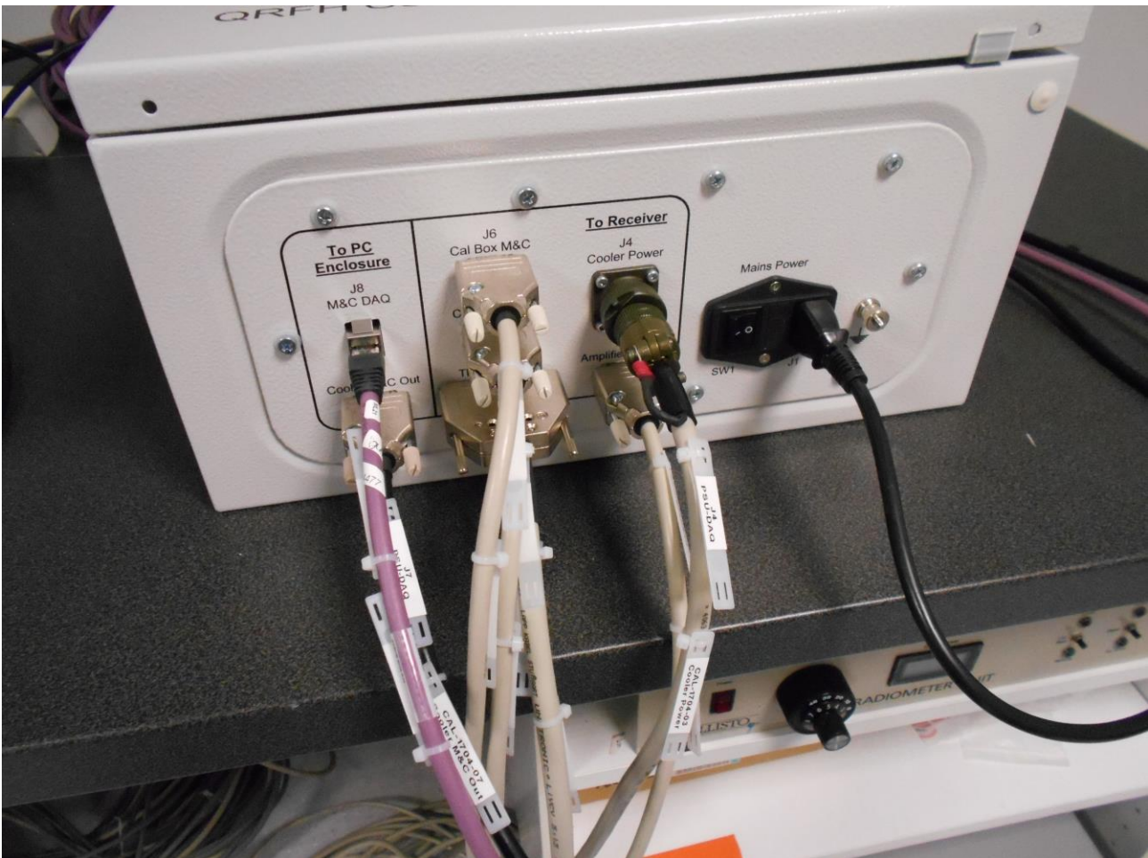
Figure 2-5: DAQ-PSU Enclosure - Cables routing space
