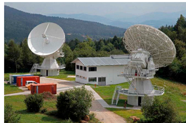
Fig. 14. Example of a VLBI2010-type antenna: the TWIN Telescope of the Geodetic Observatory Wettzell.
